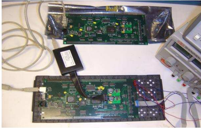
Figure 4. DSP Controller for IEM
