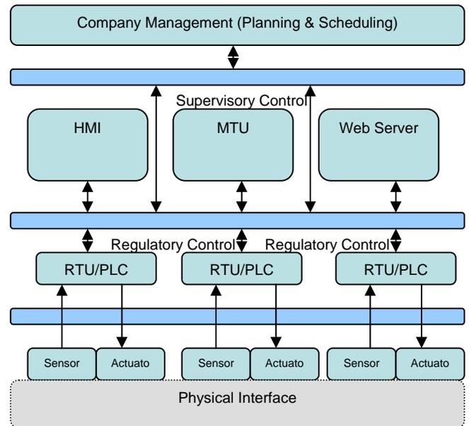
Figure 1: Reference architecture of a SCADA system
