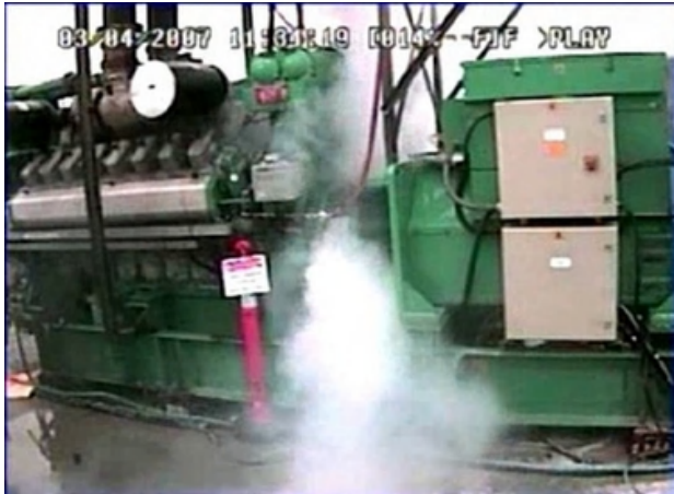
Figure 5 INL Demonstration of Destroying Large Equipment via a Cyber Attack
